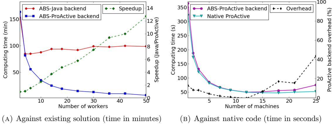
FIGURE 10. Execution time of DNA-matching ABS application
