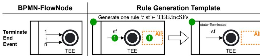
Figure 16: Rule generation template for terminate end events
