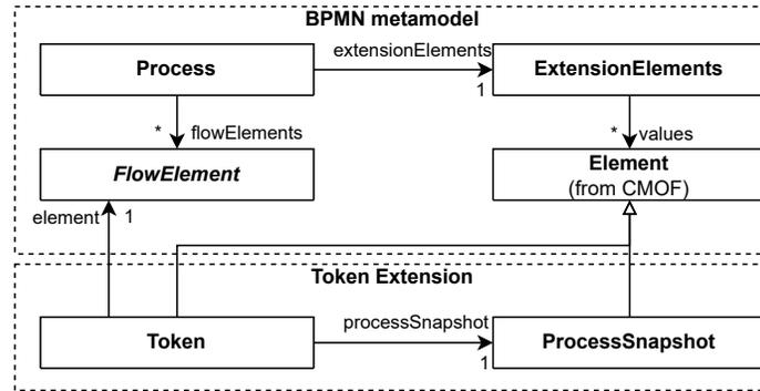
Figure 25: Token Extension of the BPMN metamodel (simplified)
