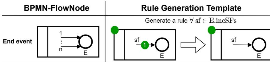
Figure 8: Rule generation template for *None End Events*
