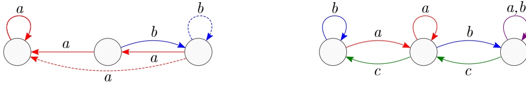
Figure 1: Two finite monotone co-Büchi automata recognising prefix-independent languages. For clarity, the co-Büchi transitions are not depicted but connect every pair of states; likewise, edges following from monotonicity (such as the dashed ones for example), are omitted. The automaton on the left recognises words with finitely many aab infixes. The automaton on the right recognises words with finitely many infixes in c(a^*cb^*)^+c .
