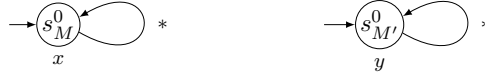
Figure 8: Two non-bisimilar systems where every computation-based strategy profile determines two different (infinite) trace outcomes, namely, x^\omega in the system on the left ( M ) and y^\omega in the system on the right ( M' ).
